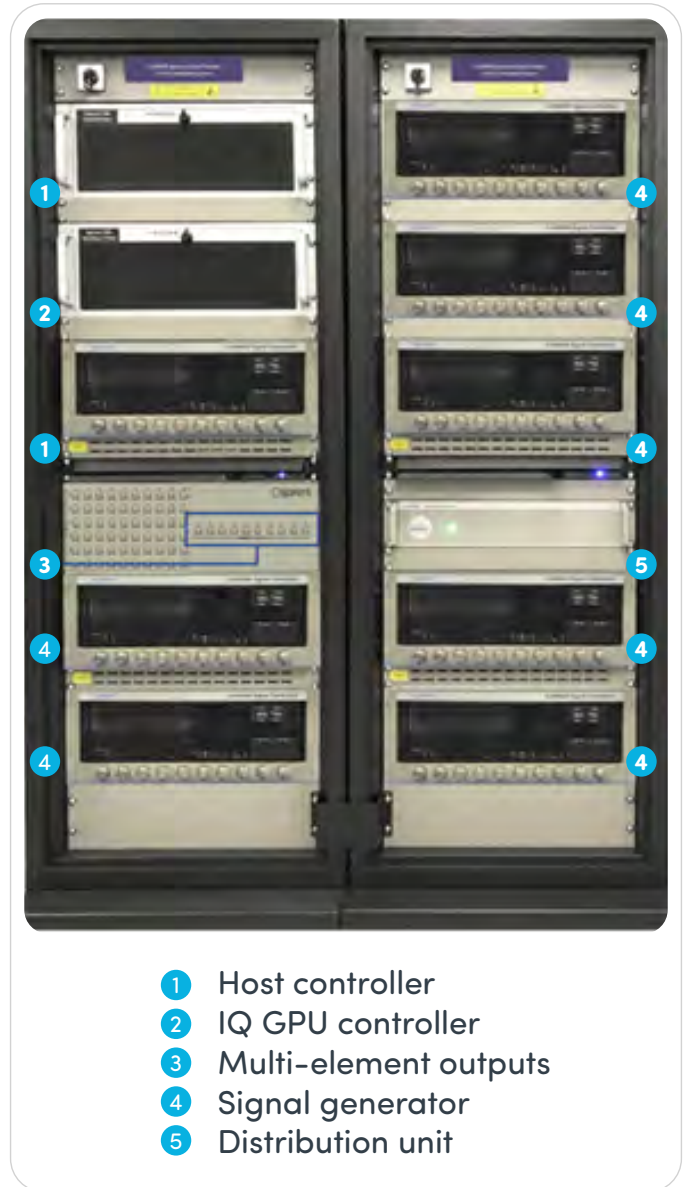
Figure 2: Example of a multi-element, multi-GNSS + jam + spoof simulation system
