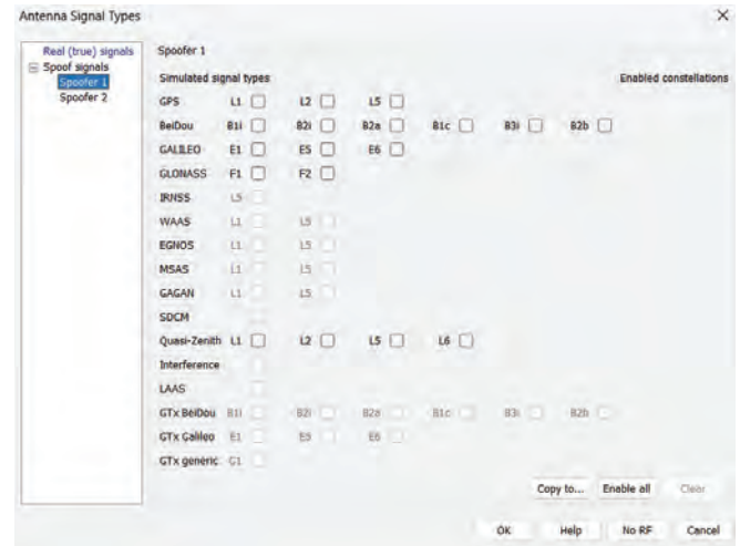
Figure 7: Vehicle antenna signal types selection Spoofers can be easily added to the scenario (see Figure 8), alongside standard GNSS constellation and vehicle groups.
