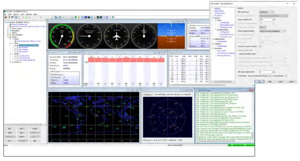
SimSENSOR™ offers complete GUI control for defining sensor parameters including sensor noise and errors such as bias and drift
